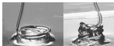
FIG. 4. Coexisting coiling states in an experiment with \nu=300 \text{ cm}^2 \text{ s}^{-1} , Q=0.041 \text{ cm}^3 \text{ s}^{-1} , d=0.15 \text{ cm} , and H=4.5 . (a) Low-frequency state; (b) high-frequency state.
